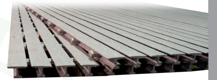
The load bars are held together using tie-bars (see picture below) and bonded with a high strength glue. The shape of the load bars, as well as the higher glass content compared to molded grating, create a stronger and more rigid grating in the direction of the load bars. Pultruded grating has uni-directional strength, as the tie-bars are not designed to carry load. Special care must be taken when designing catwalks, platforms, and stair tread to orient the load bars in the correct direction.
